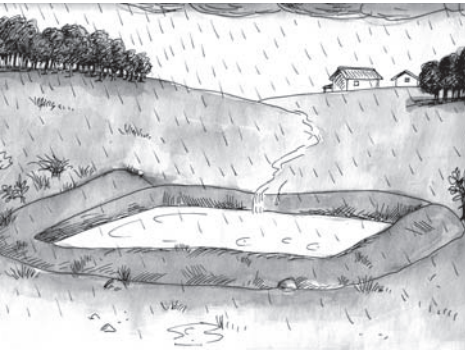
FIGURE 5 A: Excavated Pond (Unlined)
